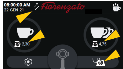
Home page with “XGi System” enabled (dosing by WEIGHT)
