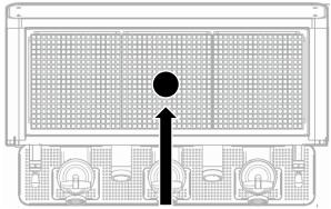
3" hole in counter recommended for passage of electrical cords & water/drain lines.
