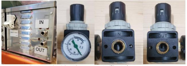
Water Line Connection Orientation: Water mains (filtration) >> IN port on pump >> OUT port on pump to IN port on pressure regulator >> OUT port to water inlet fitting on machine
